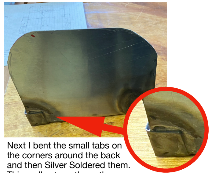
Battery tray that has been bent (except for the lip). I bent the main bend by clamping the sheet over a 2 x 4 in a vise and used a mallet to bend it. Then I bent the tabs up using sheet metal tongs.
