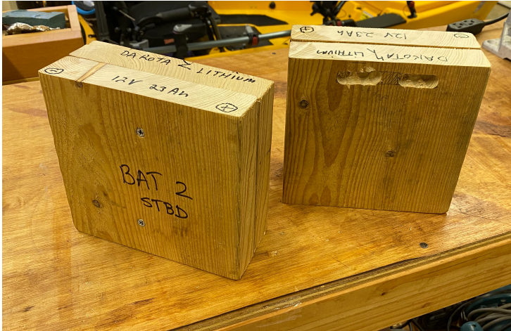
Wooden models of the batteries were made using two 6.5 inch pieces of standard 2 x 8's screwed together. Batteries are 7.125 in long x 3.03 in wide x 6.57 in high.
