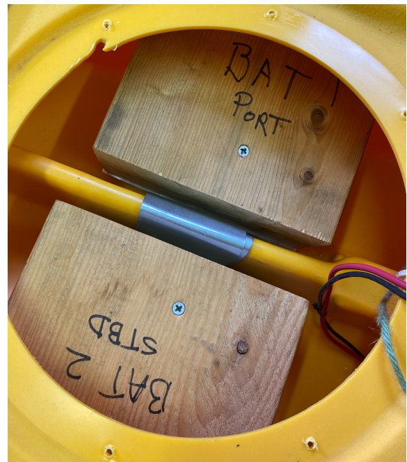
The fit was acceptable but the trays were too flimsy. A stronger lip was needed and the whole tray needed to be more rigid.
