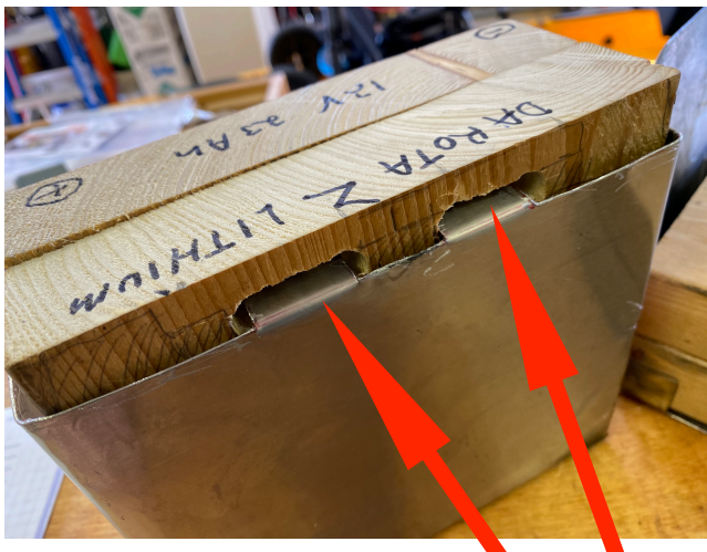
The two tabs on the front edge of the tray fit into slots on the battery case and prevent lateral movement of the battery.
